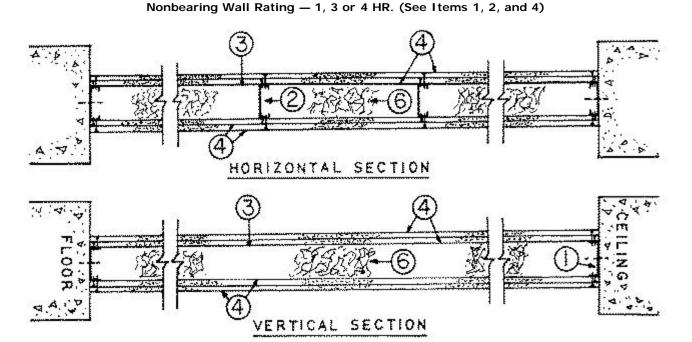
1. **Floor and Ceiling Runners** — Channel shaped 1/2 in. deep by min 3-5/8 in. wide, No. 25 gauge painted or galvanized steel. Min. No. 18 MSG for the 4 hour rating. Secured with 3/4 in. long concrete fasteners spaced 18 in. OC. For the 1 hour rating, width may be reduced to 2-1/2 in. to accommodate the 2-1/2 in. wide studs.
